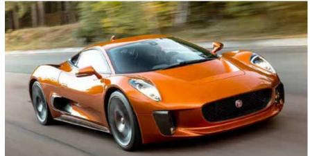
Williams Advanced Engineering to work up an alternative solution: a 1.6-litre turbo and supercharged 4cyl with e-boost to deliver 850bhp, 31 miles of EV running and a 200mph top speed.
