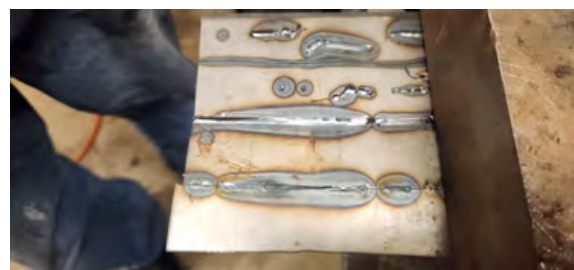
Figure 6: Note how smooth and flat the weld is - the reverse side showed great penetration
