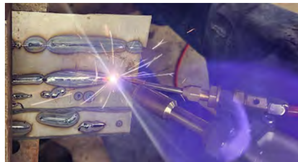
Figure 5: laser welding with wire feed
