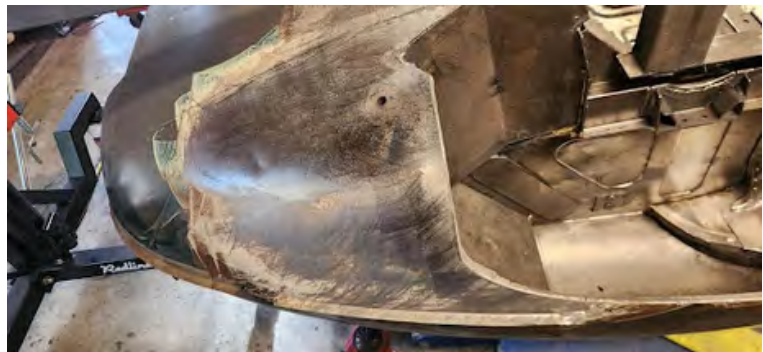
Figure 4: rear fender after cleaning - note bare metal in wheel well from previous laser cleaning
